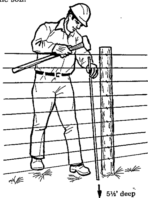
Installing a ground rod.
